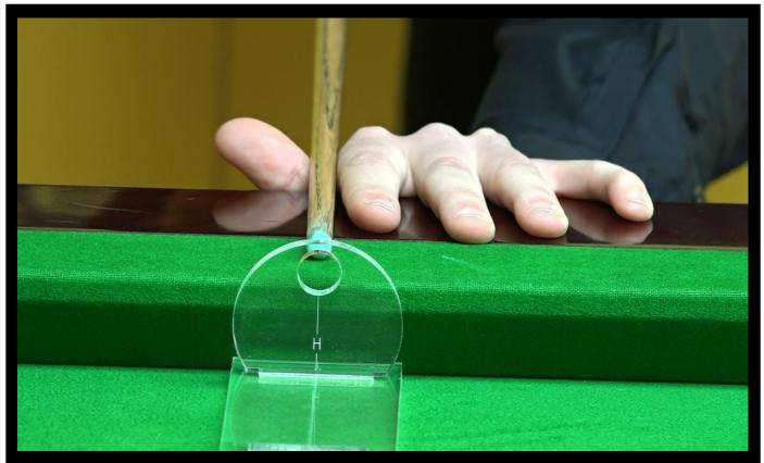
Place the Master Doctor Kit base against the cushion with part H and attempt to deliver the cue through the device to ensure a smooth delivery action.
